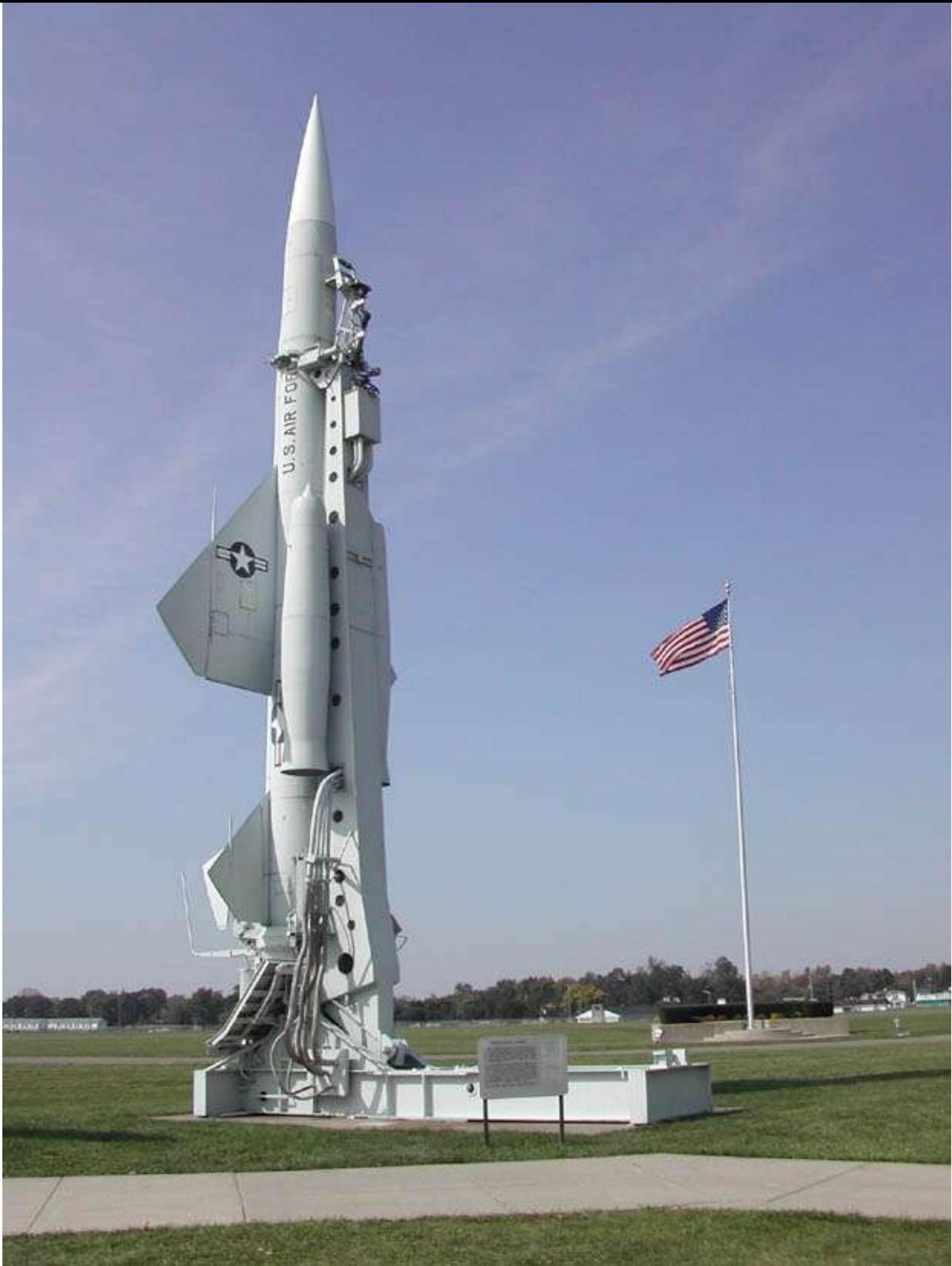
*A USAF CIM-10A Bomarc missile preserved at the entrance of the US Air Force Museum at Wright-Patterson AFB. This active guided ground to air missile of the sixties boasted a 250 NM range and could reach a target up to 60 000 ft. It was fitted with a modular 7 to 10 kt nuclear warhead.*
