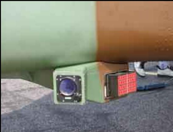
*MBDA's Saphir M CFD mounted on the helicopter boom beside the antennas of the MILDS AN/AAR-60 pointing away from the helicopter flanks at 45°. The Saphir M contains two standard NATO 32-cartridge pods, as used on the NH-90 TTH.*
