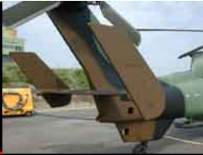
*The RWR antennas mounted on both sides of the tail fin of the Tigre have a 45° coverage. Developed by Thales Systèmes Aéroportés, this device covers the frequency bands E to K*
