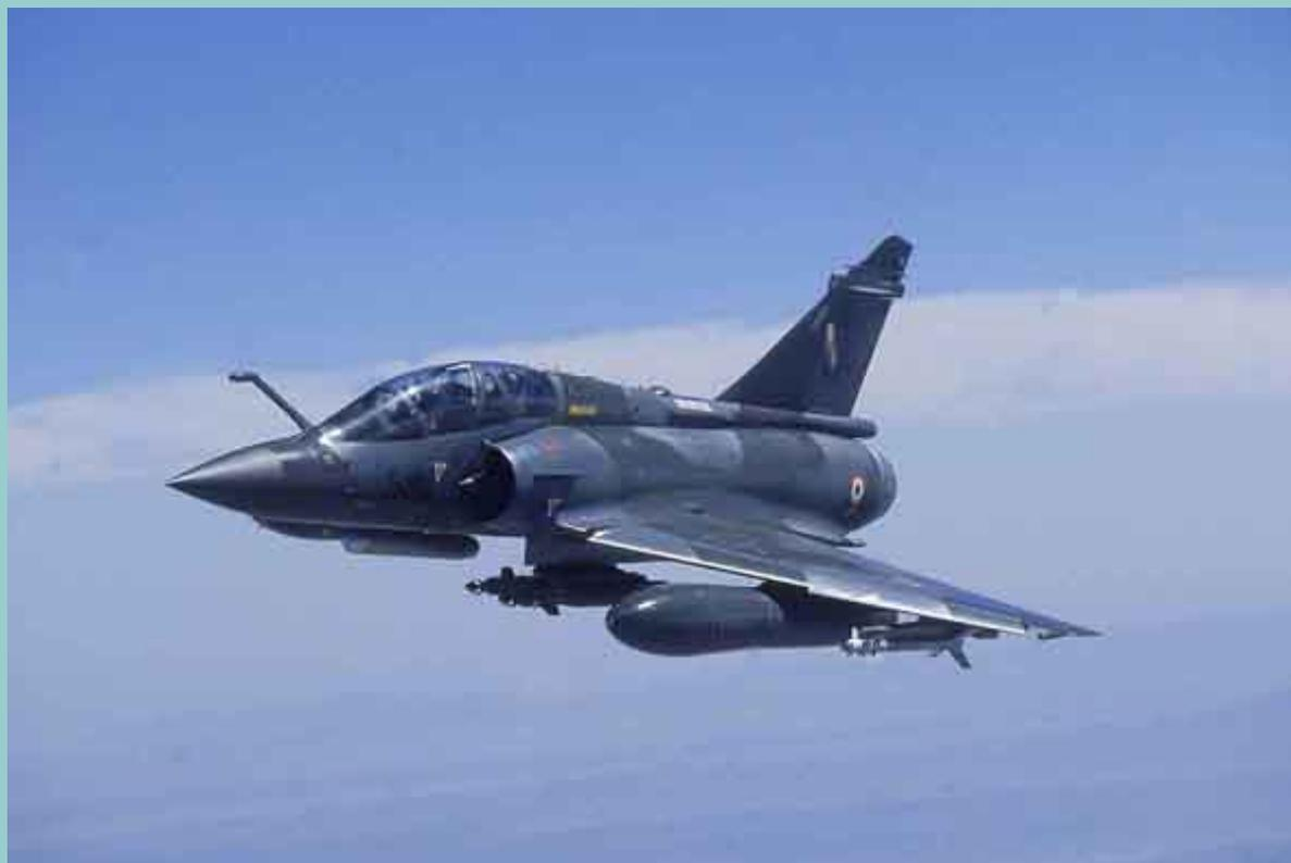
*A French Mirage 2000D fighter-bomber operating out of Ganci AB, Kyrgyzstan, in support of US-led operation Enduring Freedom against Taliban hide-outs in Eastern Afghanistan. The aircraft carries a full self-protection EW suite designed by Thales and MBDA*
