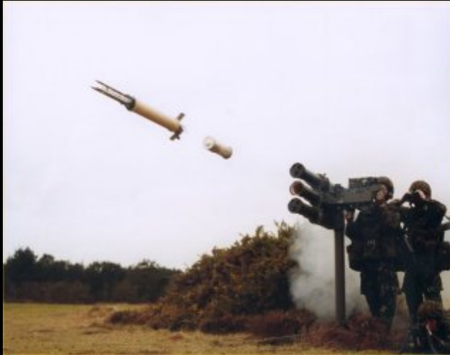
Le Starstreak (Thales Air Defence), exemple de missile sol-air laser "beam rider"
